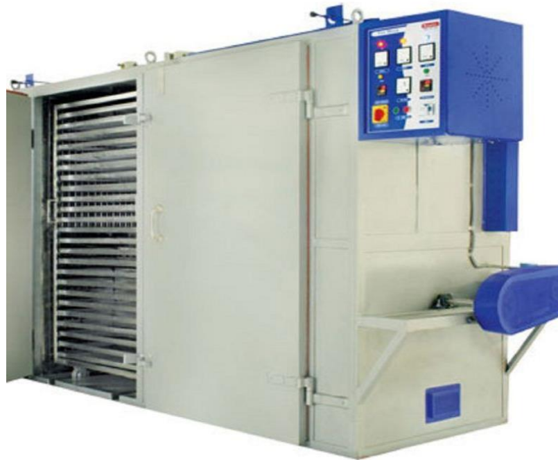
Vacuum Tray Dryer Simple, labor intensive, long drying times. Potential for encrustation/poor uniformity. Post-treatment often required.
